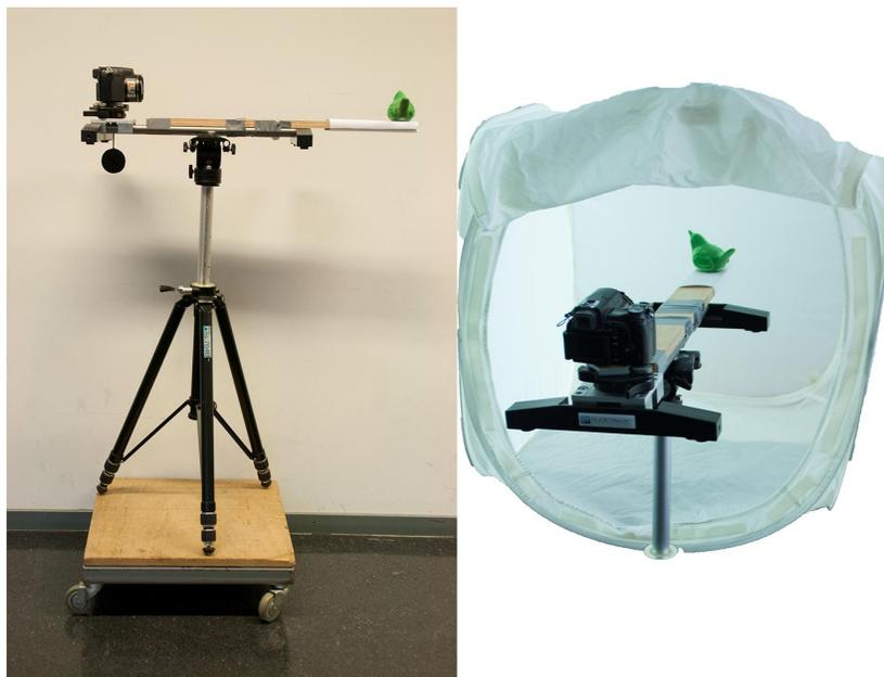
Figure 1. The setup for the photography of the object under different lighting conditions. Left: The object and the camera were fixed onto a frame attached to a tripod and placed on a small trolley. This setup could be rolled into the three canonical lighting setups of which one is shown on the right. The ambient lighting scene was created using a white photo tent – which was almost closed during the photography.
